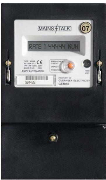
Energy monitors are only compatible with LED meters that have an **electronic display** similar to the above images. They will not work with any other style of electricity meter.
